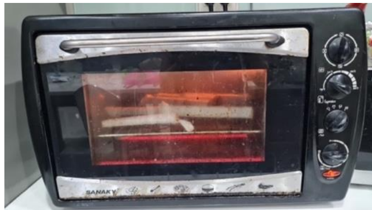
Figure 13. Heating molds with a home oven
